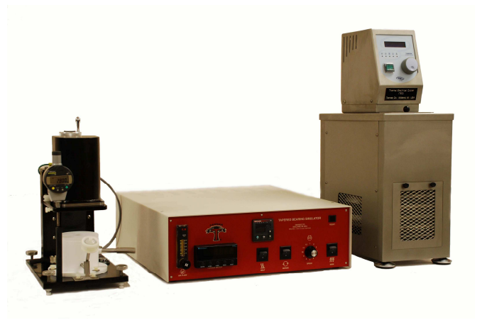
Manual Mode of Operation with Thermal Electrical Cooler (TEC) for operating at temperatures to +40°C.
